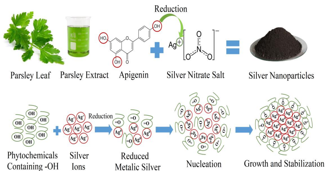
Figure 3.1. Proposed mechanism of the biosynthesizing Ag NPs from parsley extract
