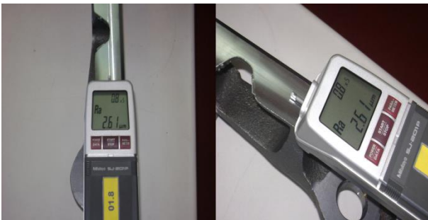
Figure 4. Surface roughness measurement on work piece
