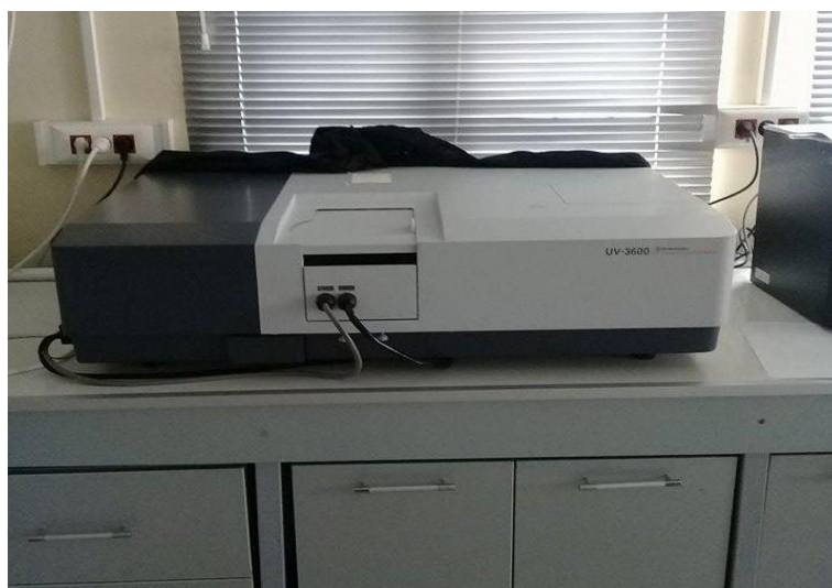
Figure 3.10. Shimadzu UV-3600 UV-VIS-NIR spectrophotometer used in our studies
