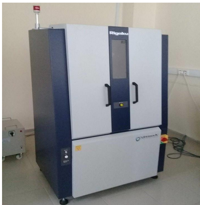
Figure 3.13. The XRD device (Rigaku Ultima IV)
