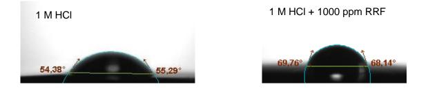
Figure 4.6. Contact angles of Cu surface after exposing to 1 M HCl solution in the absence and presence of 1000 ppm RRflower
