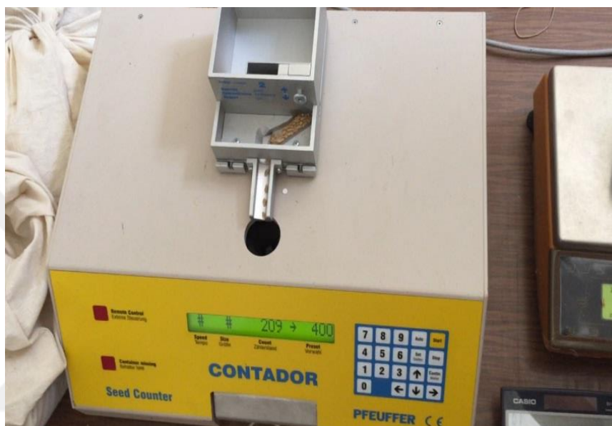
Figure 3.8. Thousand kernel weight measured by machine seed counter contador
