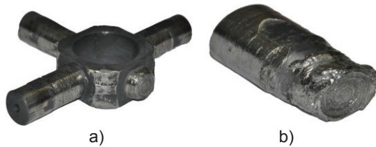
Figure 8. Broken Spider Shaft (a, b)
