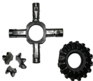
Figure 5. Broken spider gear and shaft
