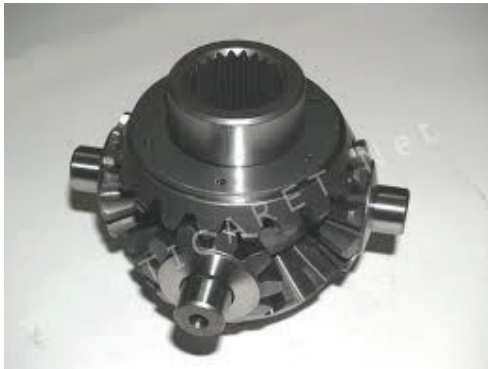
Figure 4. Axle and spider gear group
