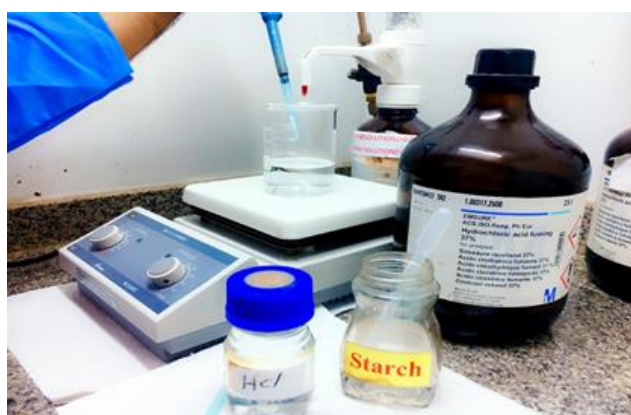
Figure 3.10. Mixture of sample with HCl ready for titration
