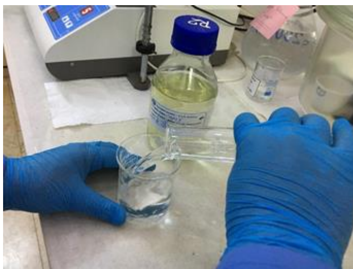
Figure 3.8. Sample dissolving with 100 mL of distilled water
