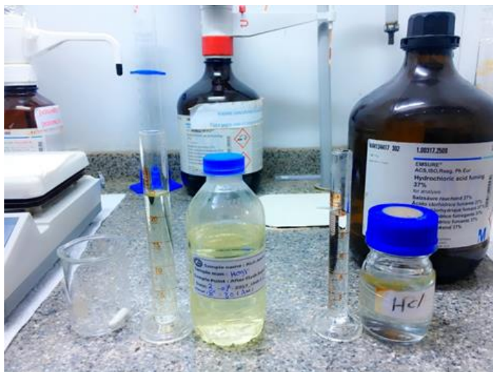
Figure 3.1. 25 ml sample with 10 ml HCl
