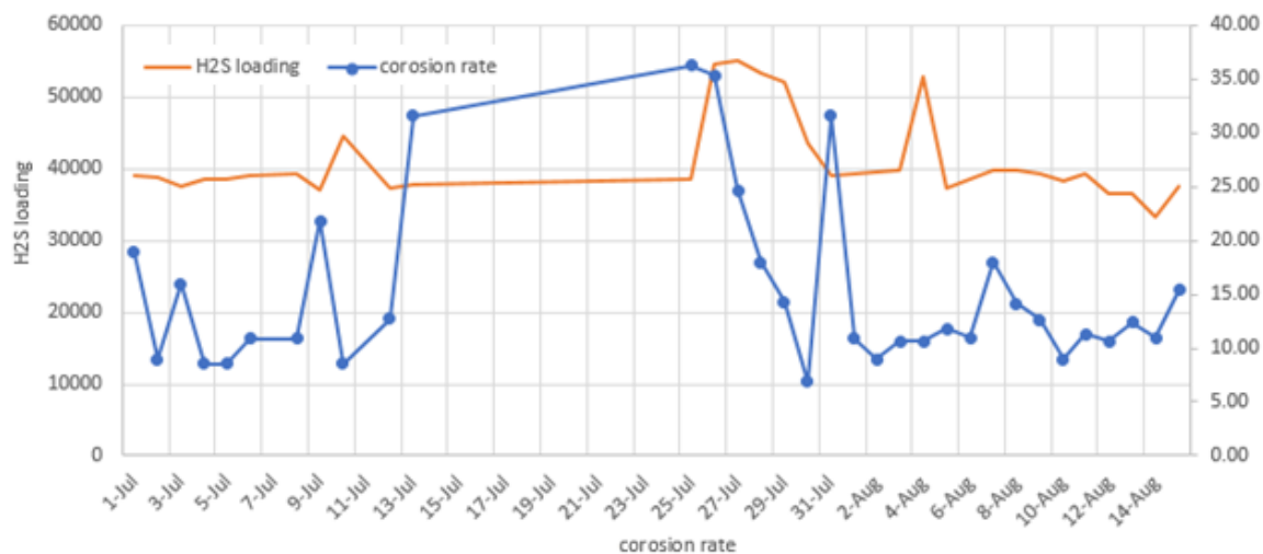
Figure 4.4. The relation between H 2 S loading with corrosion rate
