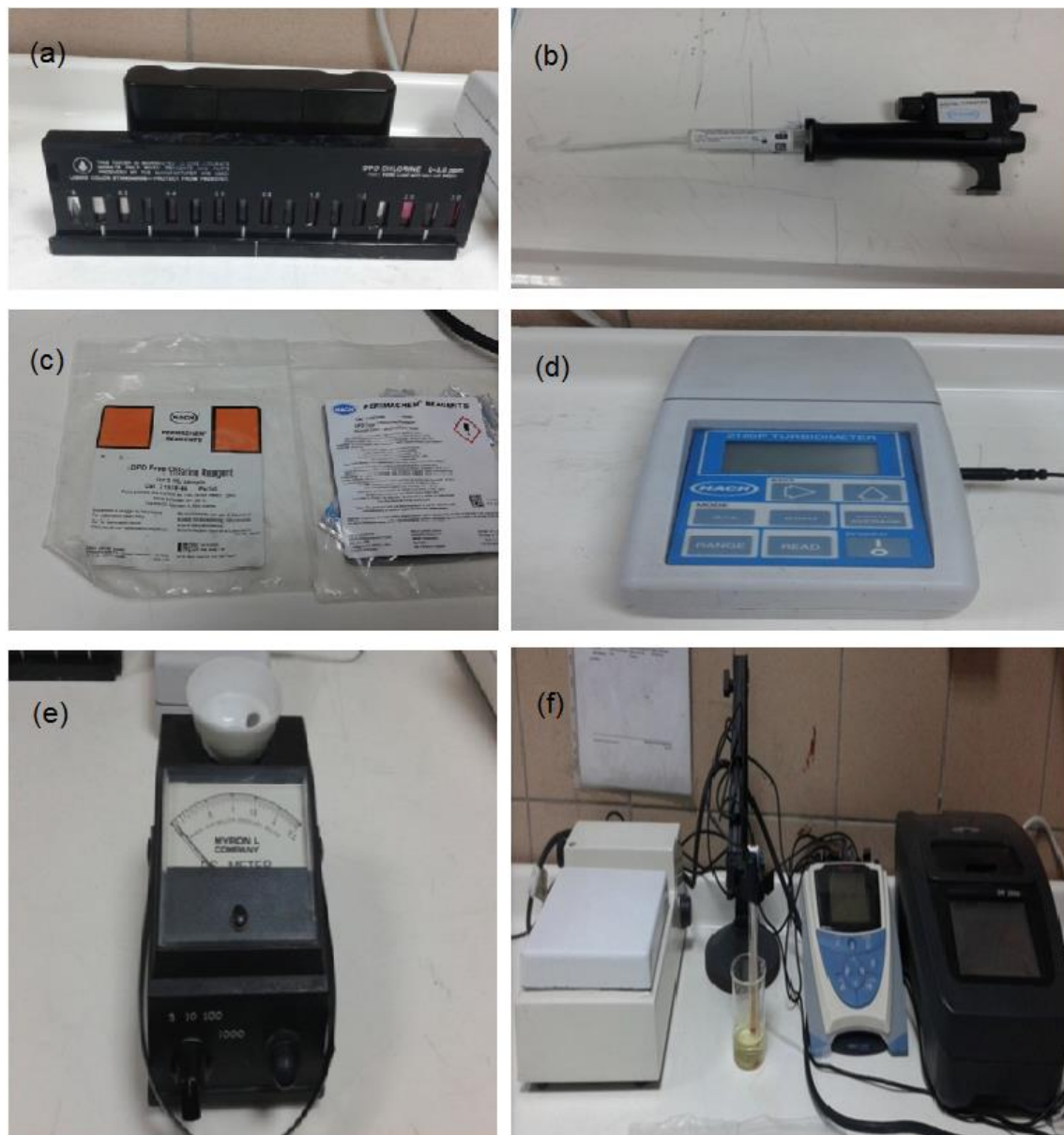
Figure 3.3. Instruments used in works: (a) Chlorine Tests, (b) Digital Titration, (c) DPD Free & Total Chlorine Reagent, (d) Turbidity meter, (e) TDS meter, (f) Thermo pH meter
